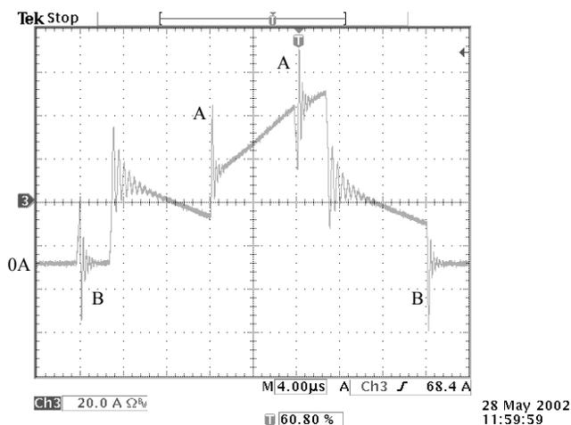
Figure 7. High Frequency transformer secondary winding current
