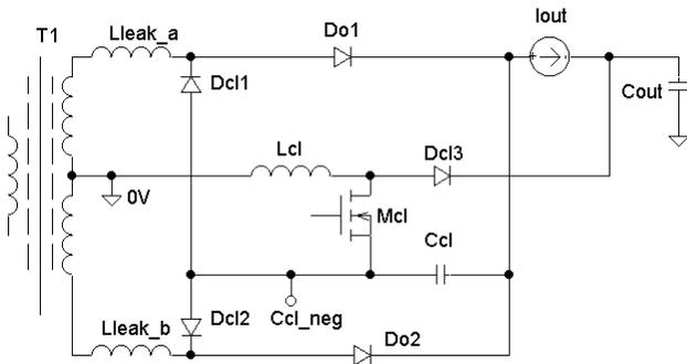
Figure 2. Basic active clamp circuit configuration.
