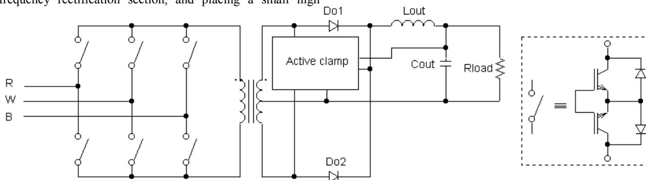
Figure 1. Three phase isolated buck converter with a secondary active clamp. AC switch realization using anti-parallel IGBT-diode combinations.
