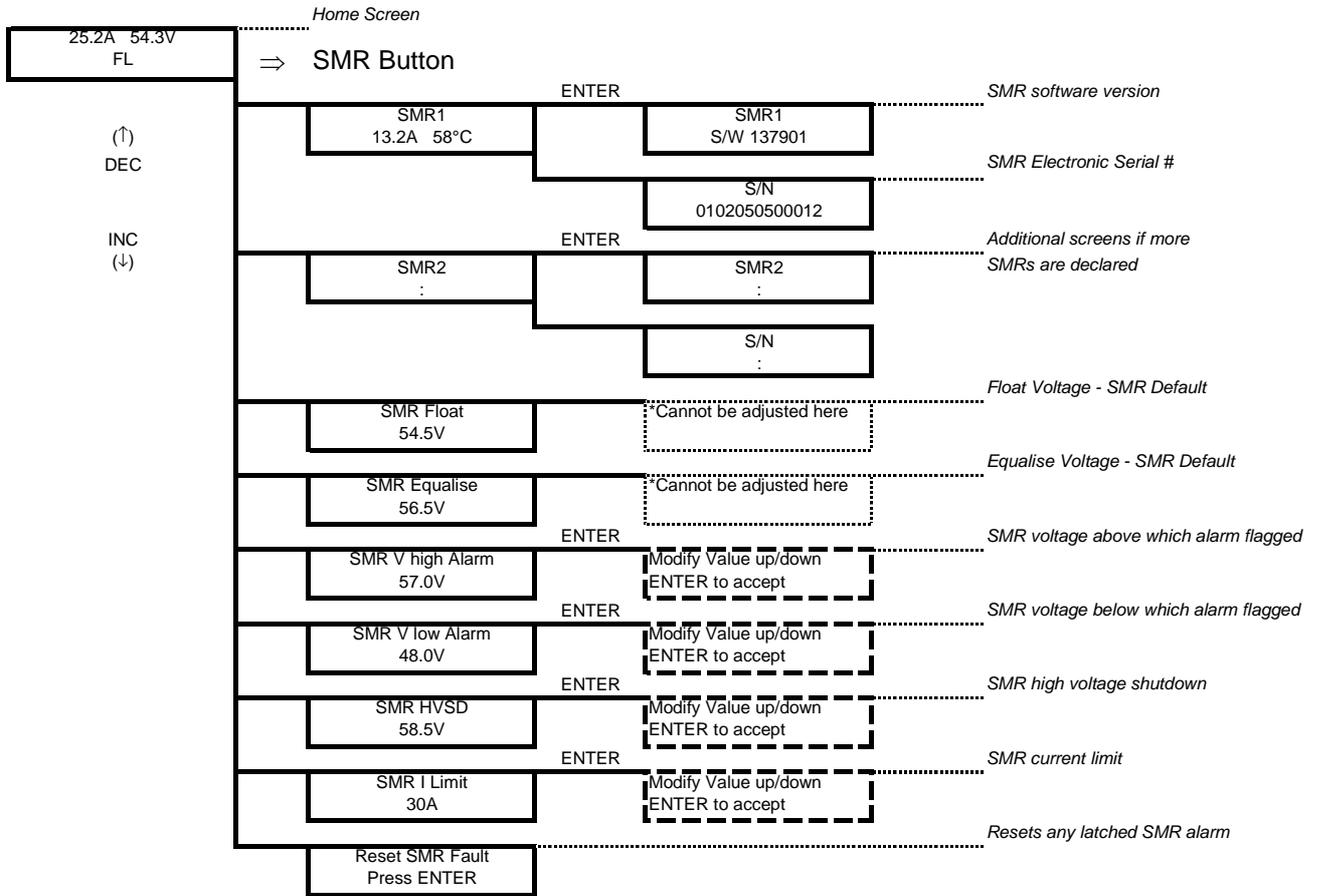
The SMR Float and Equalise voltages are the default values set in the rectifier that will be used if the MiniCSU-3 fails to operate. They are a copy of the raw values set in the BATTERY menu without battery temperature compensation and system drop adjustments.
