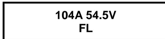
**Whenever there is no push-button activity for more than one minute, the display always reverts to this home screen. Note: the examples shown are for 48V systems. After a further 5 minutes the screen goes into a screen saver mode that is disabled when either an alarm occurs or a front panel button is pushed.**
