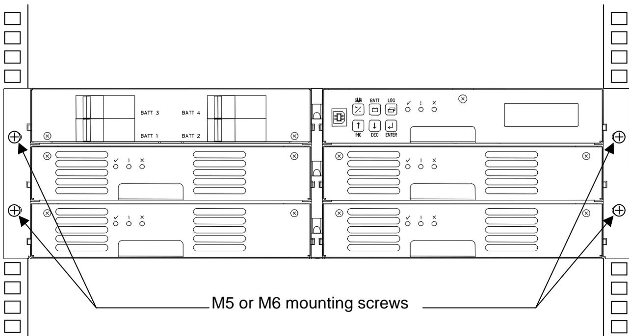
**Figure 3.1 Mount points for securing Powershelf in a rack**
