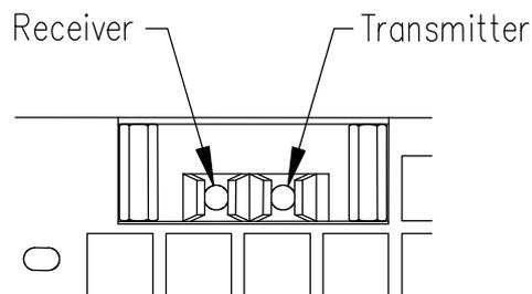
**Figure 3.14 Fibre optic connector assignments**
