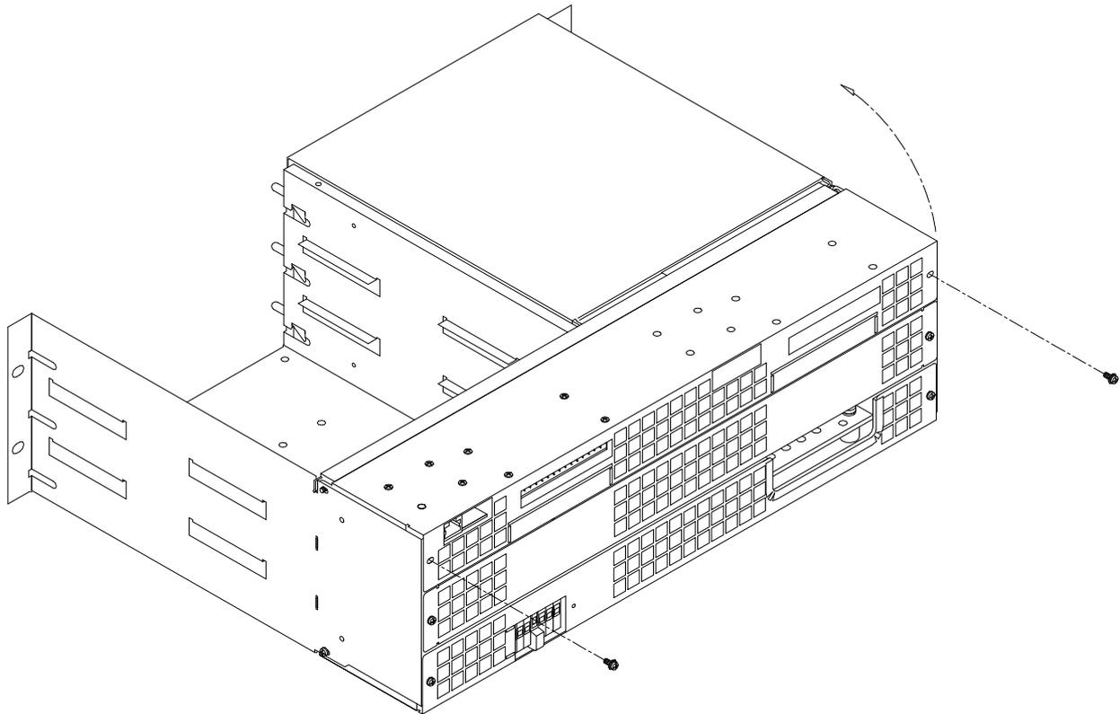
**Figure 3.2 Opening top rear cover to access wiring**
