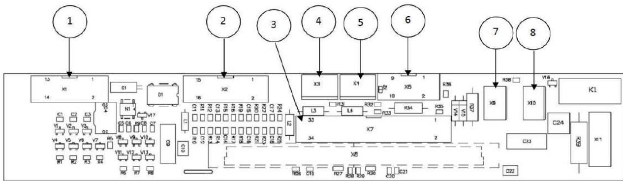
**Figure 2.4 Connections on MiniCSU-3 backplane**
